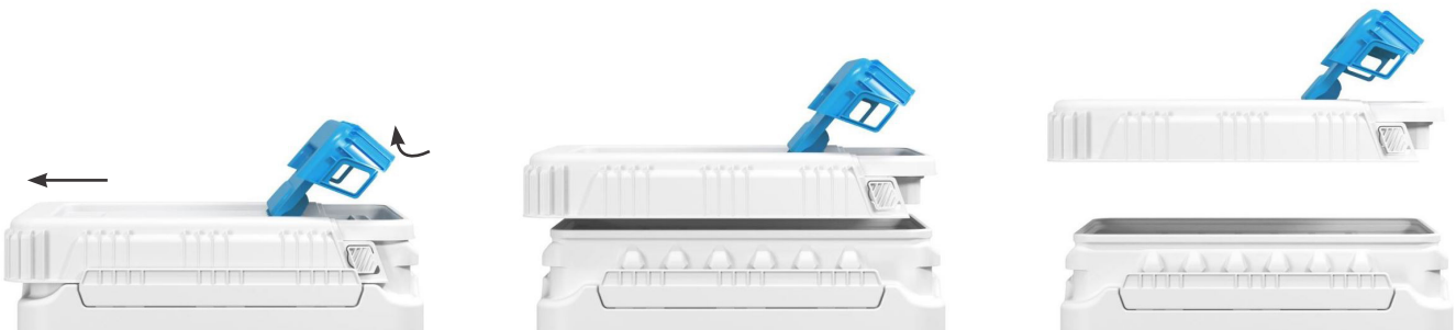
Opening of lid with sliding mechanism
